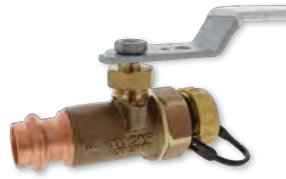
S-585HP-LF-HC Two-piece lead-free ball valve w/hose cap Full Port, 1,000 PSI CWP Solder end, stainless trim Reversible handle, triple-sealed stem Sizes 1/2" and 3/4" Page 15
