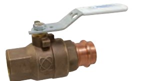
TPC-585-80/66-LF Lead-free ball valve Full port, 250 PSI CWP Threaded x press ends Sizes 1/2" thru 2" Page 21, 22
