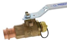
PC-585-80/66-LF-HC Two-piece lead-free ball valve w/hose cap Full Port, 250 PSI CWP Sizes 1/2" and 3/4" press end w/ 3/4" hose connection Page 27, 28
