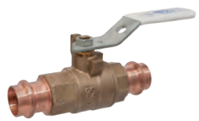
PC-585-80/66-LF Two-piece lead-free ball valve Full port, 250 PSI CWP Copper press ends Sizes 1/2" thru 3" Page 19, 20
