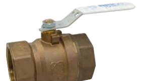
T/S-580-80/66-LF Two-piece lead-free ball valve Conventional port, 600 PSI CWP Threaded or solder ends Sizes 1-1/4" thru 3" Page 23, 24
