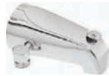
Diverter Tub Spout with Handshower Outlet Pull Up to Divert 5-1/4" Total Length w/Handshower Outlet Slip onto 1/2" C.W.T. Thread onto 1/2" or 3/4" IPS Nipple For Tub-Only or Handshower-Only Applications
