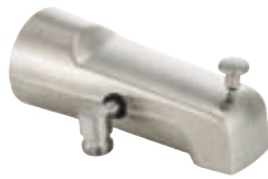
Diverter Tub Spout with Handshower Outlet Pull Up to Divert 6-1/2" Total Length w/Handshower Outlet Slip onto 1/2" C.W.T. Thread onto 1/2" or 3/4" IPS Nipple For Tub-Only or Handshower-Only Applications
