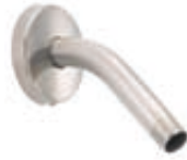
Shower Arm and Flange 1/2" IPS Male Threads 6" Long 2-3/8" Outside Diameter
