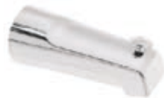
Diverter Tub Spout Pull Up to Divert 6-1/2" Total Length Slip onto 1/2" C.W.T. Thread onto 1/2" or 3/4" IPS Nipple
