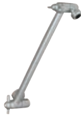
10° Adjustable Shower Arm Adjustable Up and Down 18" Brass Construction 1/2" IPS Female Inlet 1/2" IPS Male Outlet
