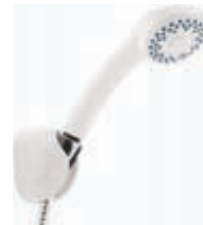
Single-Setting Handshower Features Touch-Clean Spray Holes 60" UltraFlex Hose Fixed Wall Mount 2.0 gpm @80 psi, 7.6 L/min @550 kPa
