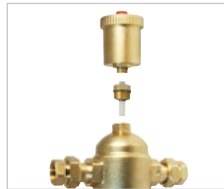
The automatic high capacity air vent attaches to the T-88 through a check valve to allow removal without system pressure loss.
