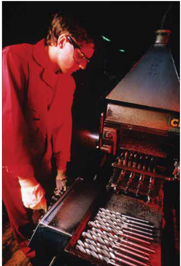
Flute milling of taper shank drills
